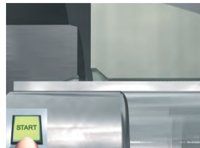
After starting the process, the dies clamp the tube and the forming pin starts to move forward
